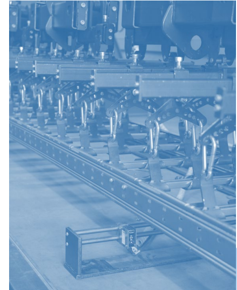
Meka Group's certified test machine to define SWL of load-bearing structures.
