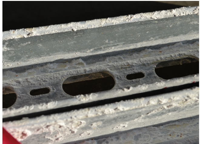
XPG® coated MEK® lighting rail after salt spray test.
