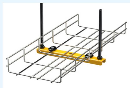
Gate support PRT is used to create E60 compliant gate supports with two threaded rods. Threaded rod GT-10 is attached to the intermediate support with two MU M10 nuts.
