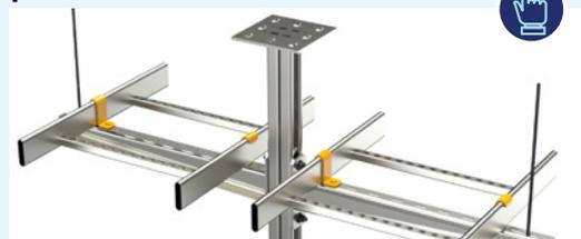
Tip attachment is required to achieve the fire rating, if wall support VK or VKF is attached with a sliding nut SMT to a mounting rail AS. In this case, a support that is wider than the cable ladder is required in order to attach the M6 threaded rod to the outermost hole.
