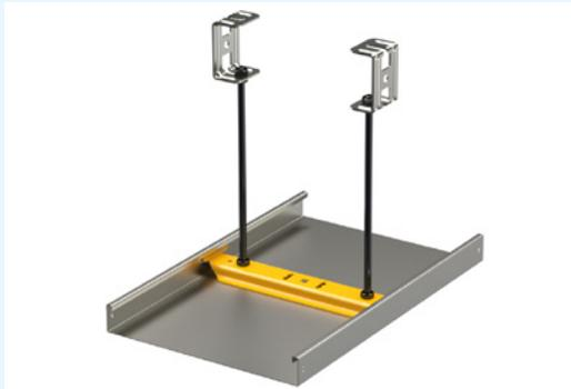
In E90 fire rating compliant gate supports, intermediate support RMK must be installed with two threaded rods. Threaded rod GT-10 is attached to the intermediate support with two MU M10 nuts.
