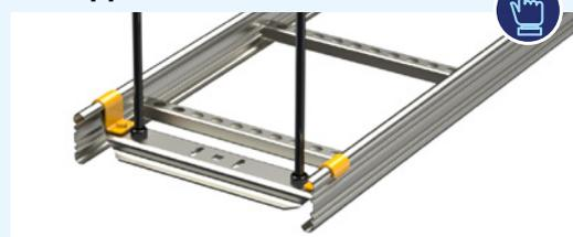
Gate supports TPK and PRT are E90 compliant, and gate support MK is E60 compliant. In an E60 compliant gate support installation, gate support MK must be attached to the ceiling with two threaded rods. Gate support MK is attached to the cable ladder with bracket KK-MK.
