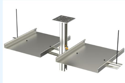
Tip attachment is required to achieve the E90 fire rating, if wall support VK or VKF is attached with a sliding nut SMT to a mounting rail AS. In this case, a support that is wider than the cable tray is required in order to attach the M6 threaded rod to the outermost hole.
