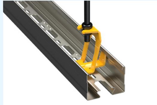
MEK lighting support rails are suspended in an E60 fire rating compliant manner with intermediate support MEK RK. The intermediate support is suspended from the ceiling with a threaded rod.
