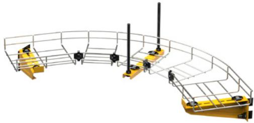
Fire rating E60 compliant 90° angles are achieved by cutting the wire mesh tray as shown in the example and joining the edges together with connector set WMT CL. The corner must be supported in the middle as well as no further than 300 mm on both sides of the corner.
