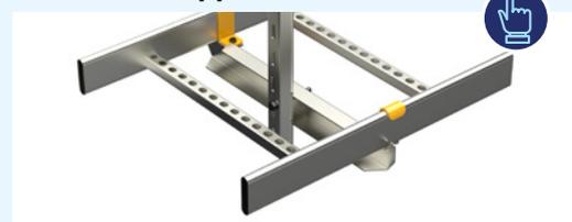
In an E90 compliant intermediate support installation, ceiling support TP1 is attached to intermediate support HK13 with screw set RS3. The cable ladder is attached to intermediate support HK13 with bracket KK.
