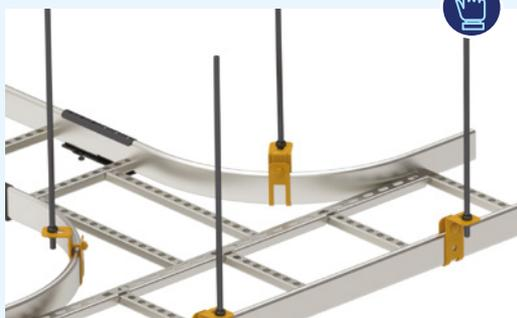
KST and KSX must be supported no further than 300 mm from both joints, or in the middle of corner, if distance to the joint is less than 300 mm. On demand, KST and KSX must be supported so that the span length of the product does not exceed the allowed span length of the concerned cable ladder when measured the length in the median line of the arc.
