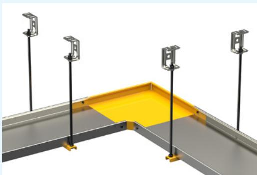
In an E90 fire rating compliant corner installation, corner piece RS90 must be supported at no further than 300 mm from both joints. Support can be done with gate support PRT. Gate support PRT must be attached to the ceiling with two threaded rods.
