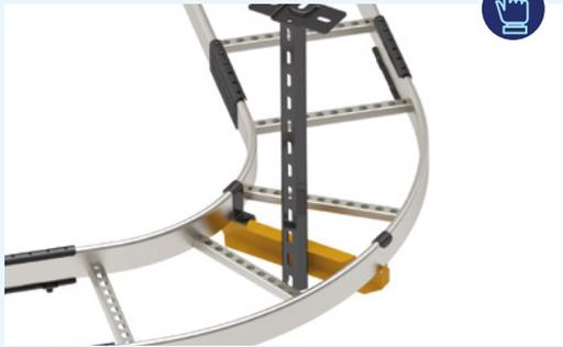
Corner piece must be supported no further than 300 mm from both joints, or in the middle of corner, if distance to the joint is less than 300 mm. On demand, corner piece must be supported so that the span length of the corner piece does not exceed the allowed span length of the concerned cable ladder when measured the length in the median line of the arc.
