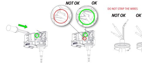
2. Check that conductors are properly installed and assemble lid by pressing it to adapter body Lid cannot be removed after assembly
