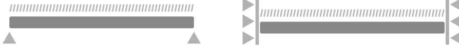
FIGURE 29 A simply supported beam on the left and fixed supported beam on the right. Both arrangements are well-known and presented in literature.
