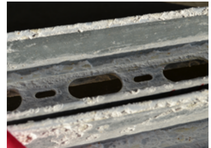
XPG coated lighting support rail MEK after salt spray test.
