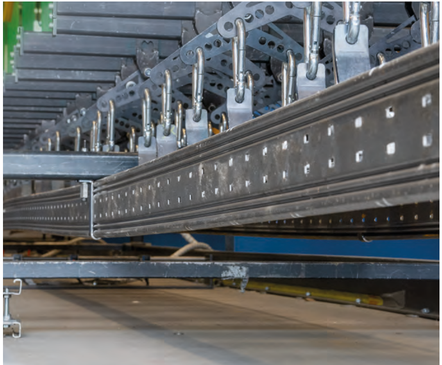
Products tested according to the standard allow the customer to compare systems with each other. The picture above shows the cable ladder being tested for the safe workload with the calibrated test device in Meka Pro's testing laboratory.
